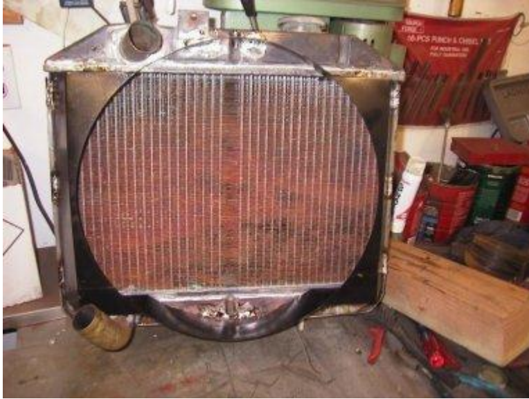
35. Shroud fitted and soldered as per original spots:
