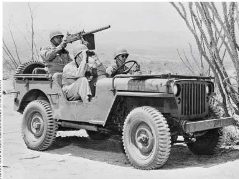
This photograph from 1942 shows three soldiers on patrol in a Jeep that has been outfitted with a machine gun, one of the offensive weapons, including rocket launchers and anti-tank weapons, that the Jeep could mount.
